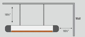
Locate stud in ceiling or wall and securely fasten bracket. Attach heater to bracket, adjust to desired position and tighten down. Must have minimum 72" clearance from the floor.
