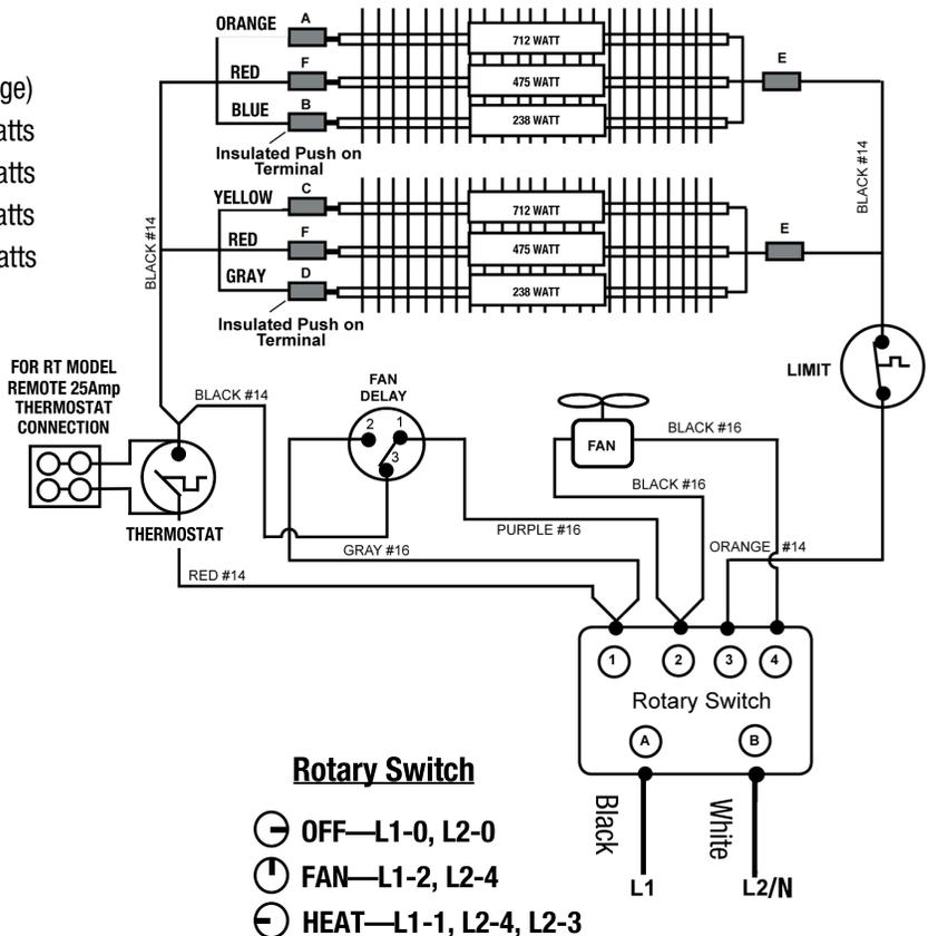
Wiring Diagram# KBP1230 120 Volt 2850 Watt unit heater
